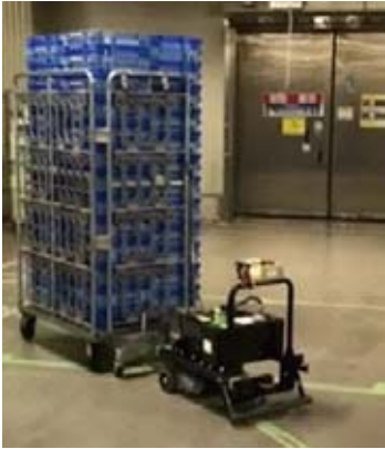
AGV for transporting roll pallets
