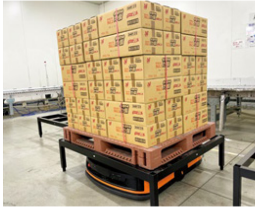
AGV for transporting pallets
