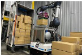
Robot loading cargo on a basket cart
