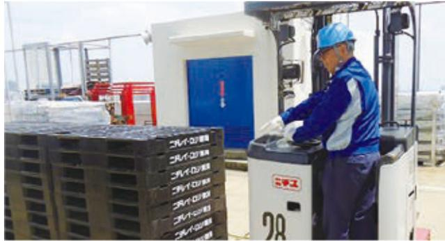
Specialized course for developing the skill of confirming safety while driving a forklift using the “point and call out” method
