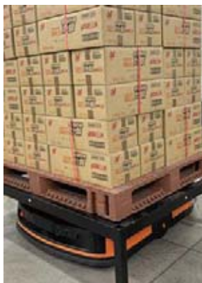
AGV for transporting roll pallets
