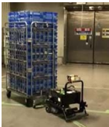
AGV for transporting pallets
