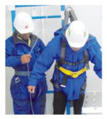
Confirming the usefulness of "falling prevention equipment" while suspended in midair
