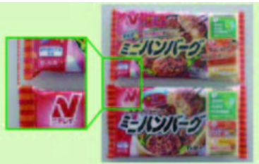
Ultrasonic sealing of plastic film packaging
